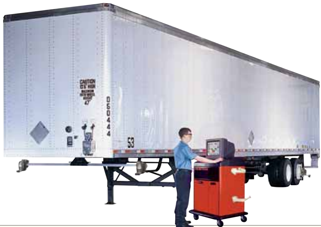
Trailer Alignment Gauge Tool (optional) mounts sensors to the trailer kingpin. Trailer axles are adjusted to centerline. Optional DSP506T-XF Sensors shown.
