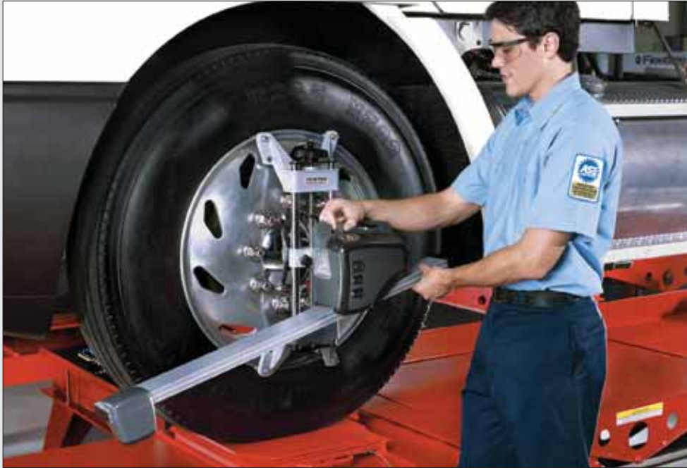
DSP506T Sensor shown here with standard Self-Centering Wheel Adaptor.
